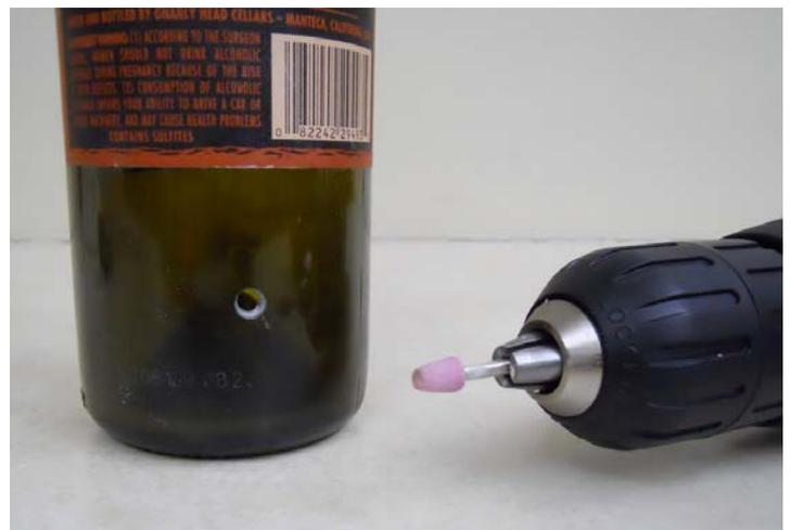
cutting through the glass. To keep it from getting too hot and avoid cracking, I keep a small glass of water next to me, dipping the drill bit into it every few seconds or so to make sure that the drill bit stays cool. Some people put the bottle in a tub of water while they drill, I don't like to do that because I don't want to ruin the label. You shouldn't have any problems as long as you keep the bit wet and don't twist the bit or push too hard.
