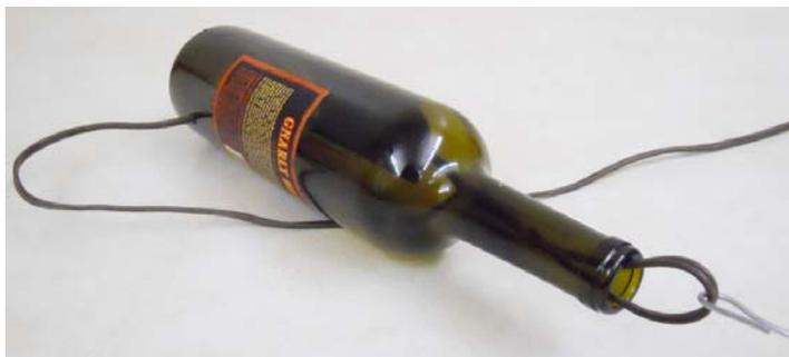
If you are having trouble getting your hole started, put a piece of masking tape on the spot where you'll be drilling, this helps keep the bit from "running away". Once the hole is drilled, **fish the cord through** the hole and up & out of the neck. You might need to use a wire hook to do this.
